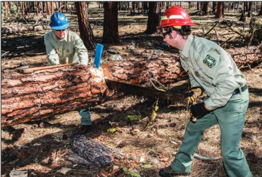
Figure 11-55—Using a wedge to hold a kerf open on a log.
