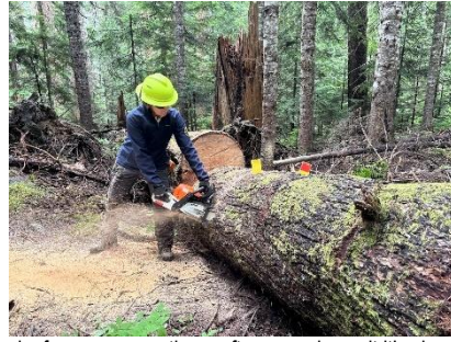
And, of course, sometimes after you release it it's close to the ground (chain dulling risk).
